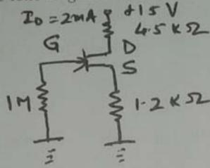
(c) Plot the output for the following circuit, if the input is a sinusoidal voltage with peak value 4V.
