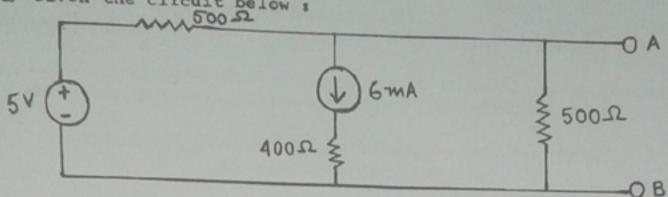
Find the open circuit voltage V<sub>TH</sub> across terminals A and B of the Theyenin Equivalent Circuit.
