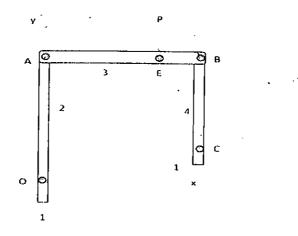
(b) Figure below shown is an indicator mechanism. The bell crank arm is pivoted at O and has mass moment of inertia 'l'. Find natural frequency of the system.
